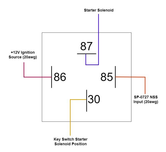
A 30AMP fuse is recommended for terminal 30 on the RELAY.
