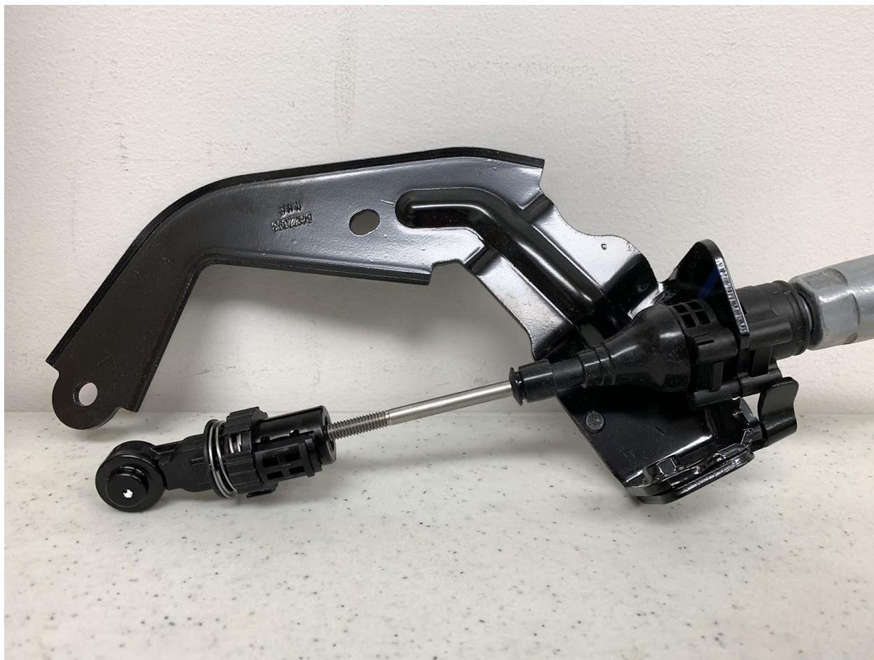
Cable attached to the transmission bracket:
