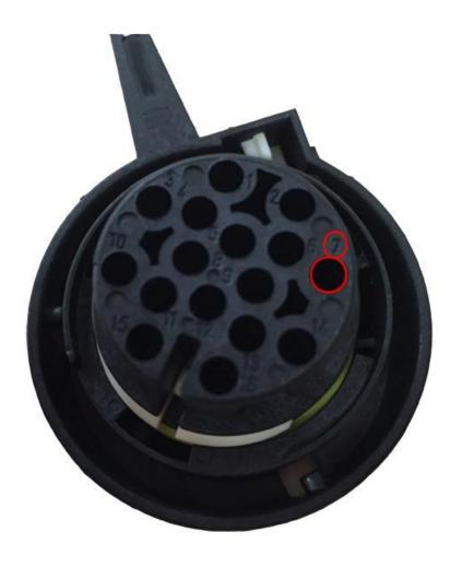
Insert our white/black wire into position 7 of the harness side of the connector.
